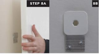
Line up the panel. Slide down until you feel the flange contact the top of the Z CLIP. Push in on the panel and slide it down to engage the Z CLIPS. Make sure all clips are engaged to complete installation.
